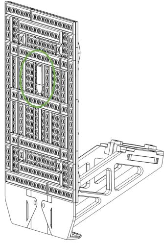
Carefully lower n. The Lego should neatly nestle into the 3D printed geometry.
