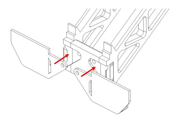
Install both screws into the back stretcher. Do not over tighten (use a screwdriver).
